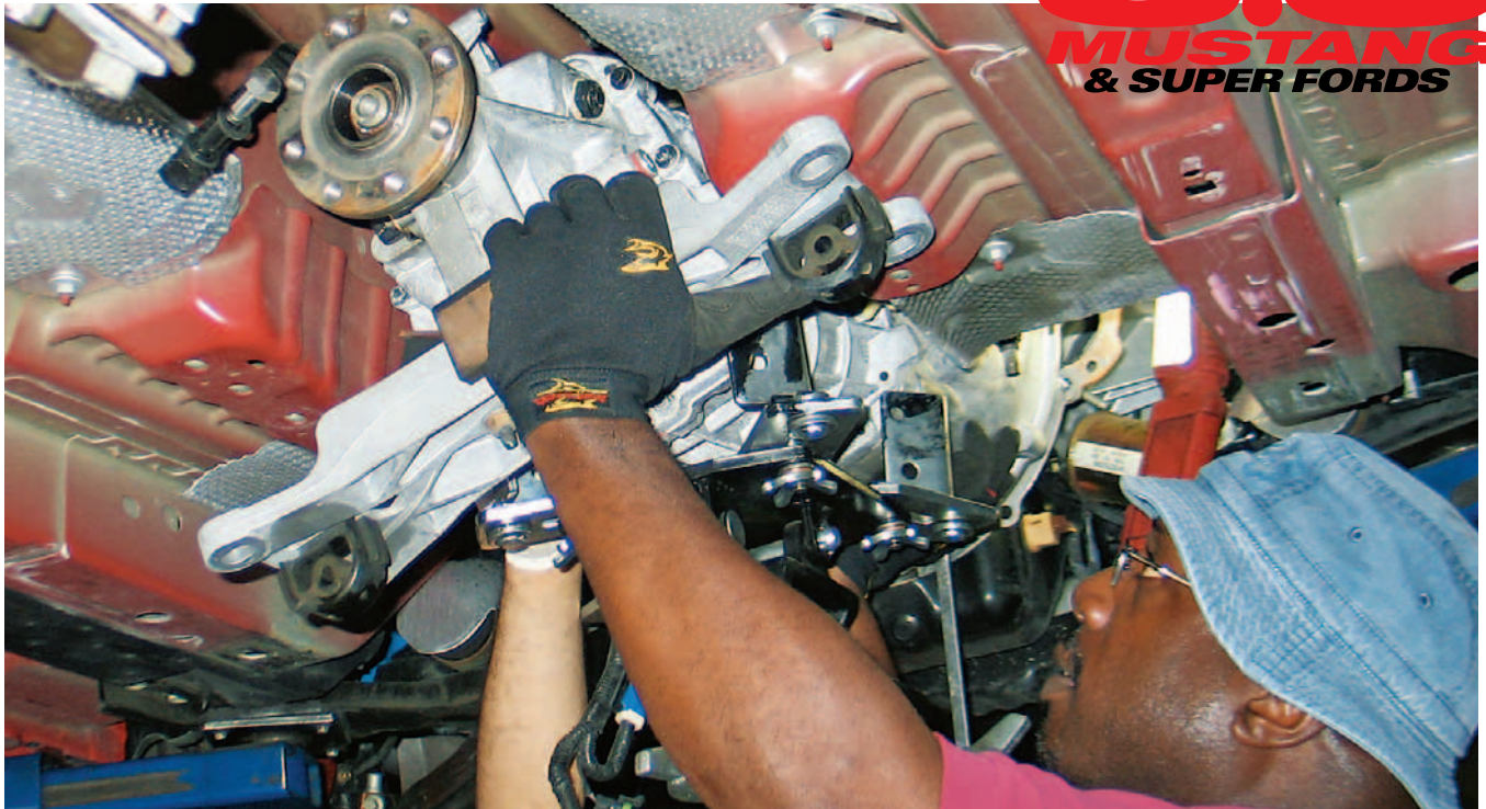
▲ Saul "The Surgeon" Gutierrez of Extreme Automotive and your tech editor stuff the Tremec TR-3650 tranny back into Chris McCollum's '05 GT after installing McLeod's new RST twin-disc clutch.
