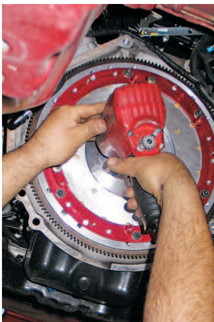
▲ With the floater's mounting ring installed, Saul sets the new aluminum flywheel in place and tightens each bolt with an impact gun. If you're working without air tools, flywheel bolts are torqued to 75 lb-ft.
