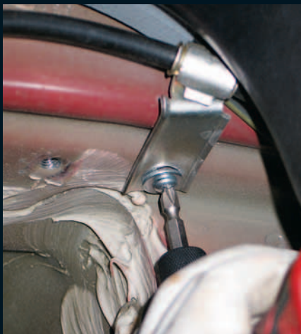
▲ Moving the emergency brake cable slightly and a few taps of the hammer on the floor near the back of the car to knock down a high spot are the only necessary chassis mods for installing the new driveshaft. When we say "taps of the hammer," we mean it. There's absolutely no need to wail on the tunnel or floor.
