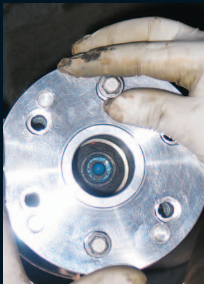
▲ Each S197 driveshaft kit includes this adapter hub for the pinion flange that allows perfect-fit installation of the shaft using factory bolts.
