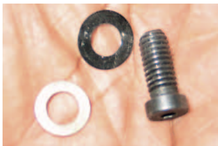
▲ This is a sample of a critical bolt and washer set. The floater ring is secured to its mount in three places using an Allen bolt and two washers at each point. Installing each bolt-and-washer set in the correct hole of the floater's mounting ring is critical, as the hardware represents weight (in grams) that can affect the clutch assembly's balance and function if the pieces are installed in the wrong place.
